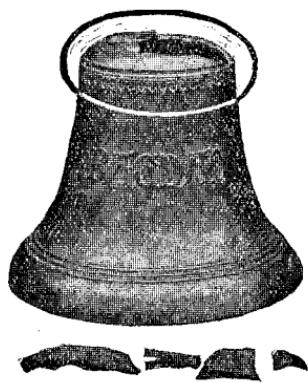
*A large Bell fractured at dome
