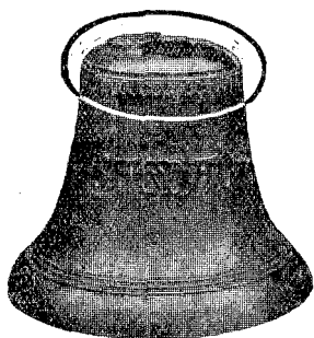
A large Bell fractured at dome and parts completely broken out.
