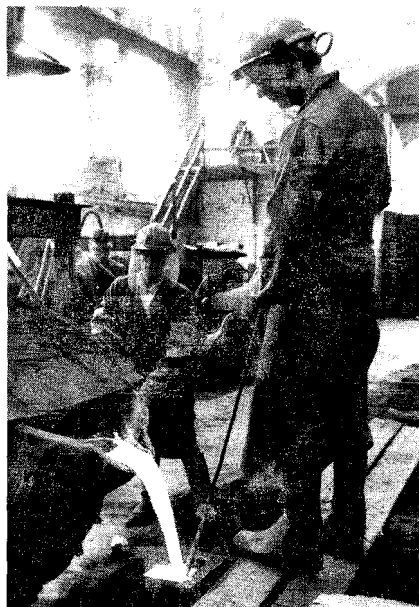
Casting the new peal of 8 bells for the Church of St Nicholas, Harpenden, Herts. June 1990.
