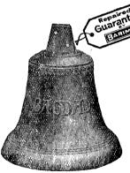
The same Bell after repair by Barimar Welding Process. Stringent tests proved that the tone of the bell was in no way affected by the welding, while the dome of the bell was much stronger than before and able to resist greater strain. The Repair was done at a small cost in THREE days and under Barimar Guarantee.
