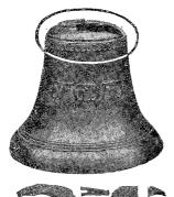
A large Bell fractured at dome and parts completely broken oul.
