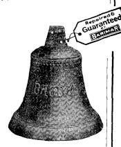
The same Bell after repair by Barimar Welding Process. Stringent tests proved that the tone of the bell was in no way affected by the weloing, while the dome of the bell was much stronger than before and able to resist greater strain. The Repair was done at a small cost in THREE days and under Barimar Guarantee.
