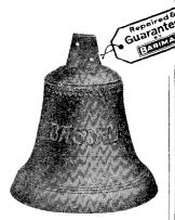
The same Bell after repair by Barimar Welding Process. Stringent tests proved that the tone of the bell was in no way affected by the welding, while the dome of the bell was much stronger than before and able to resist greater strain. The Repair was done at a small cost in THREE days and under Barimar Guarantee.
