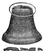
A large Bell fractured at dome and parts completely broken out.
