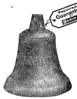
The same Bell after repair by Barimar Welding Process. Stringent tests proved that the tone of the bell was in no way affected by the welding, while the dome of the bell was much stronger than before and able to resist greater strain. The Repair was done at a small cost in THREE days and under Barimar Guarantee. No. 357.—IPSWICH (St. Mary-le-Tower Society).—On Saturday, November 19th, 1927, in three hours and thirty-three minutes, at the Church of St. Mary-le-Tower.
